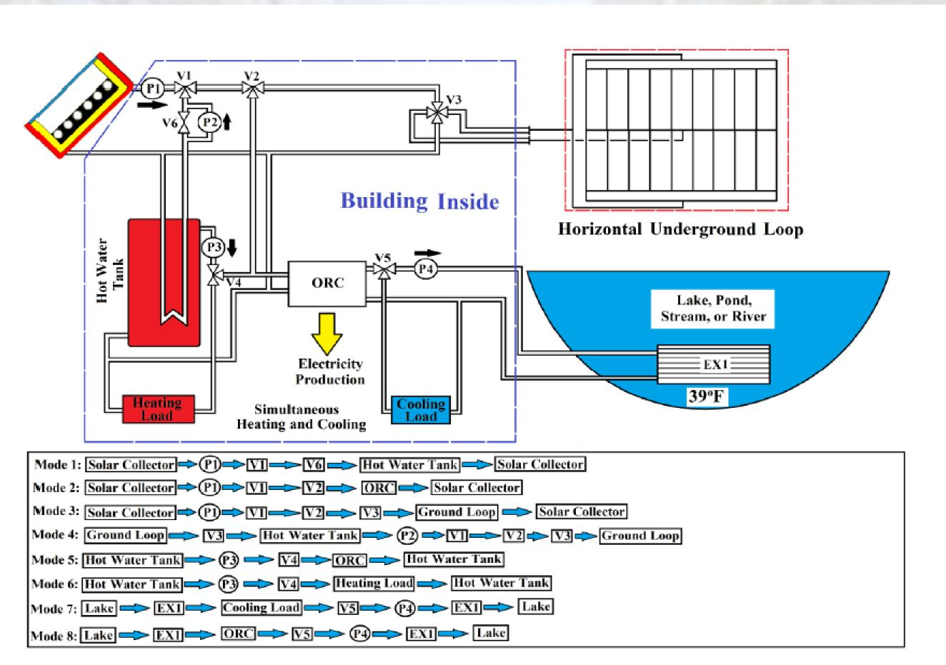
Figure 3: HVAC System with Seasonal Storage and Electricity Generation
