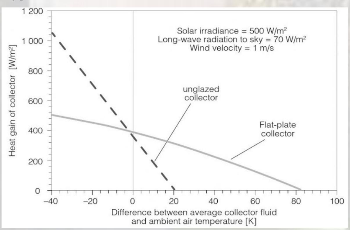
Fig. 1: Solar Thermal Collector Performance (Hadorn et al., 2015)
