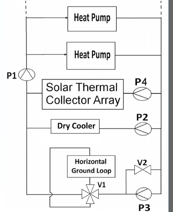
Figure 2: Hybrid or Multi-source Heat Pump System
